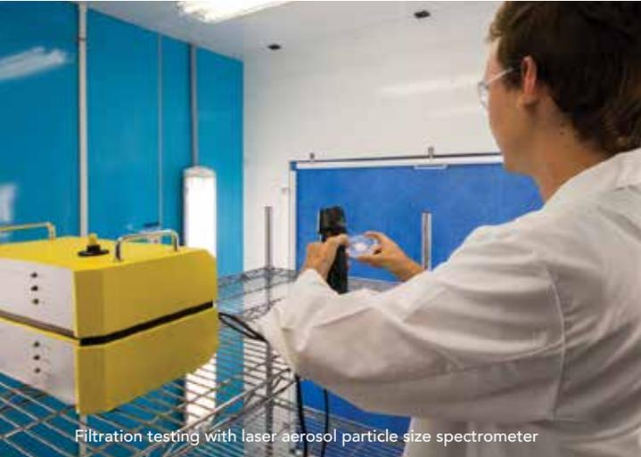
Filtration testing with laser aerosol particle size spectrometer
