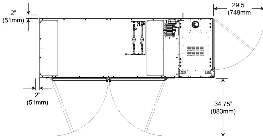
Figure 2-1 Installation Clearances
